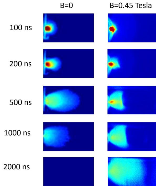
Figure 5.7 Images of barium plasma in the absence and presence of different magnetic fields.
