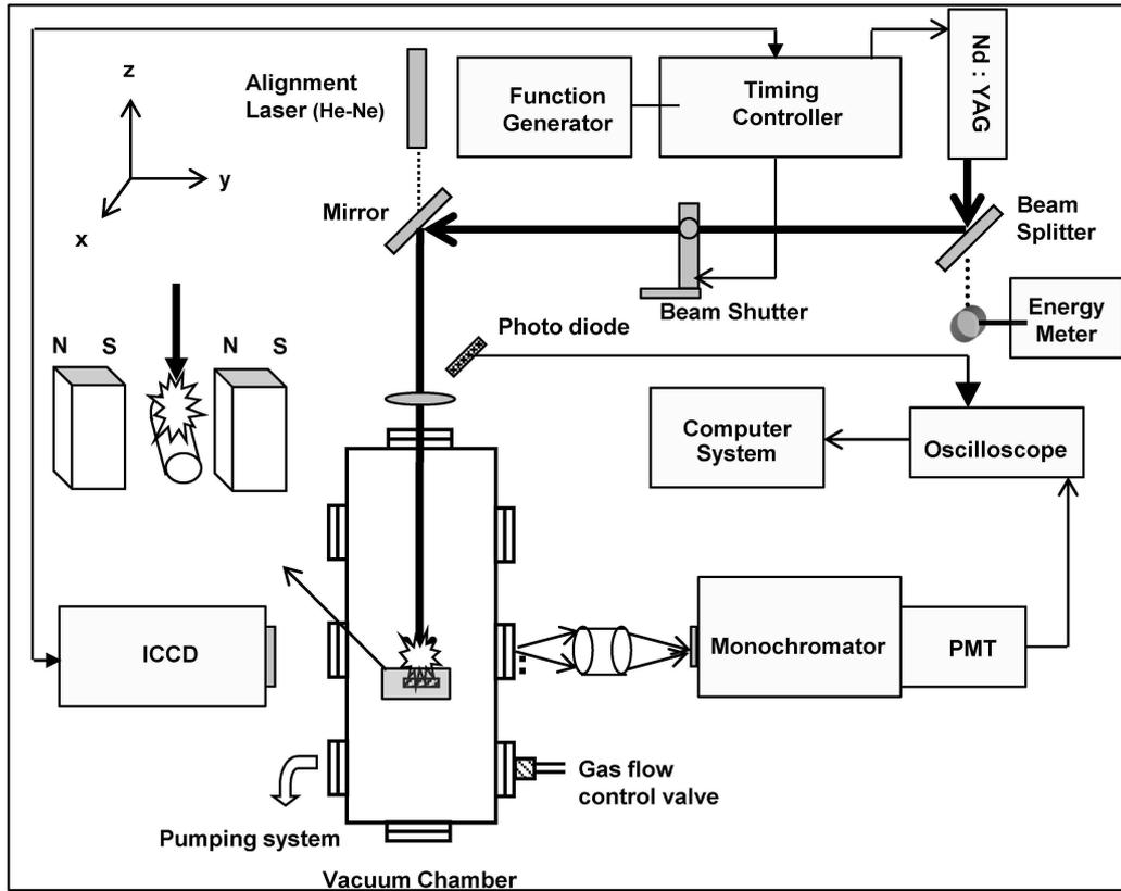
Figure 2.5 Schematic of the experimental setup
