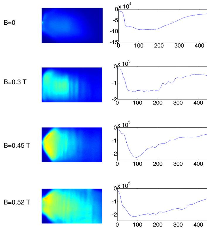
Figure 5.3 Intensity variation at different magnetic fields
