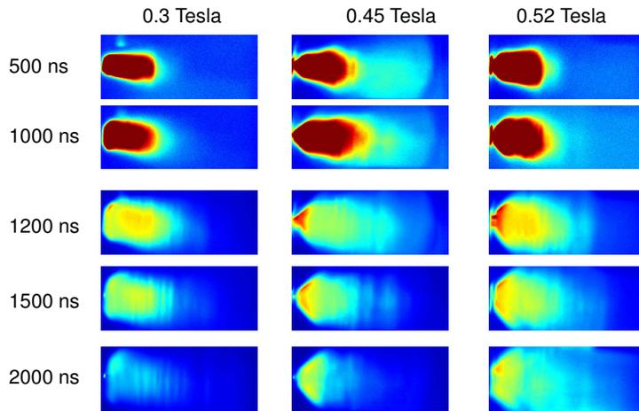
Figure 5.2 Images of tungsten plasma at different magnetic fields
